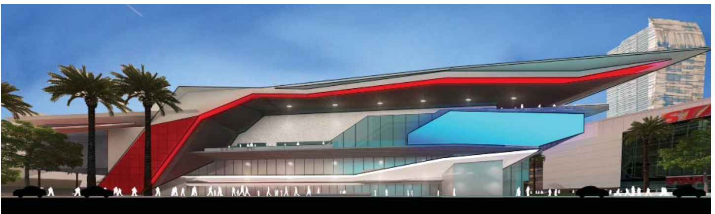
Above: An elevation drawing of the new ballroom and meeting room complex shows how the structure will cantilever over the walkway by Figueroa Street.
